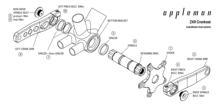
NOTE: Grease all surfaces that touch each other during installation or use. Grease entire spindle surface including lobes and bearing surfaces Grease threads, under bolt heads, all metal mating surfaces etc... Proper greasing will ensure durability and maintainability of the cranks. BONUS: pinch bolts, retaining ring, spindle bolt threads have factory grease applied.
